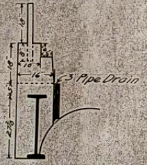
Detail of parapet, guard rail and drain.
